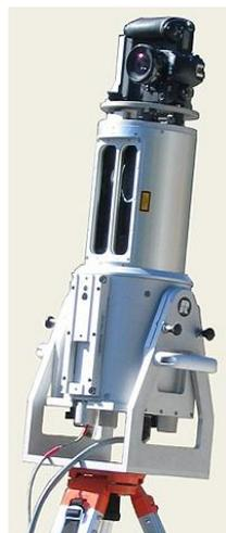
Figura 3 – *Laser scanner* 3D RIEGL (ARTESCAN)
